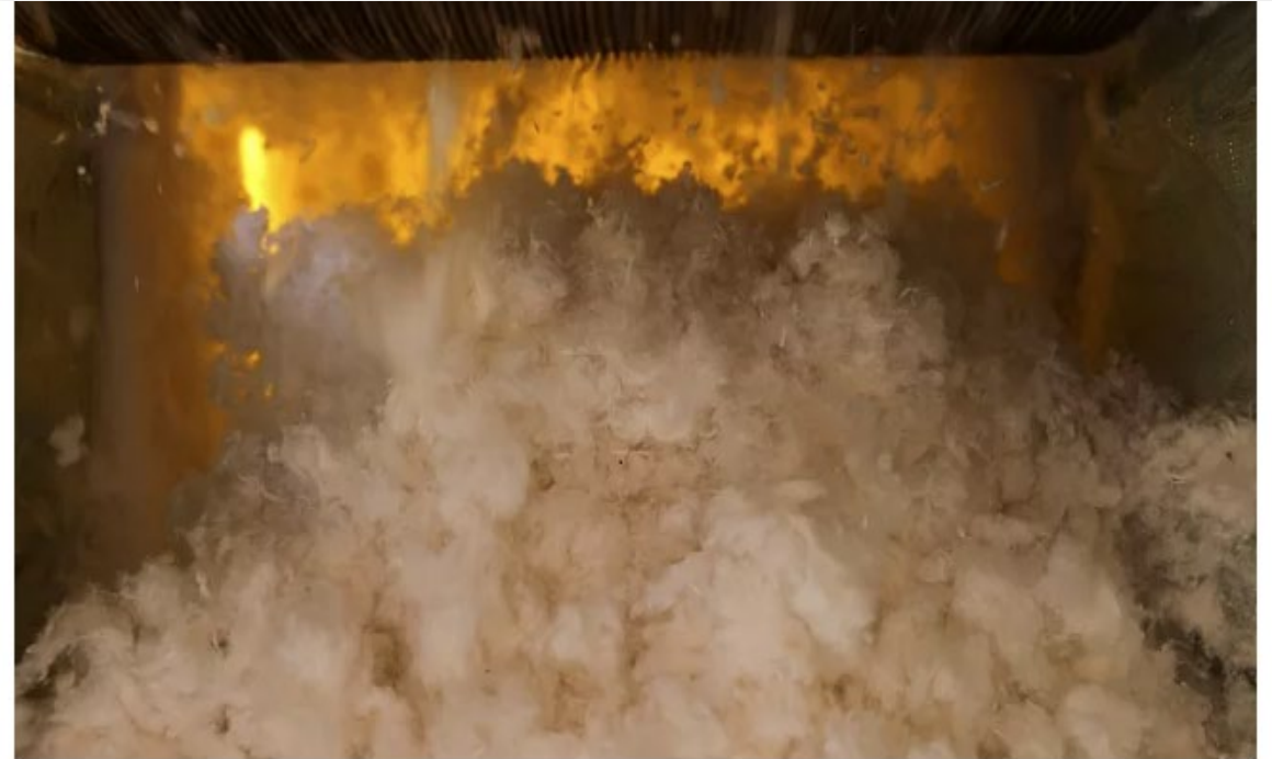
Recycled fibre made from cigarette filter tips is seen in a cotton gin machine at a cigarette butt recycling factory in Noida, India. - REUTERS/Anushree Fadnavis
